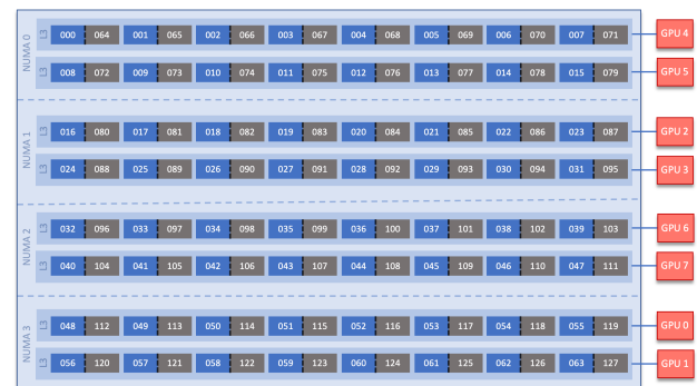
Figure 2: OLCF Frontier simplified node diagram [30]. Note that the GPU indexing [[4, 5], [2, 3], [6, 7], [0, 1]] is non-intuitively associated with the NUMA domain ordering [0, 1, 2, 3].
