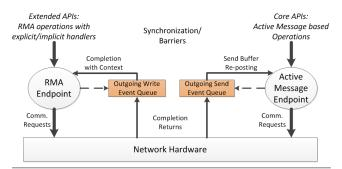
**Figure 3.** GASNet over SFI: two endpoints for RMA operations and Active Message based operations, respectively, with separate Event Queues for completions.
