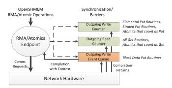
**Figure 2.** OpenSHMEM design over SFI: a single endpoint is used for RMA/Atomics operations, with Event Queue for block put routines and Counters for other operations.
