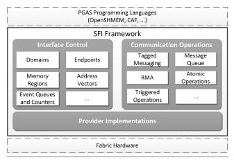
Figure 1. Architectural View of Scalable Fabric Interface Framework
