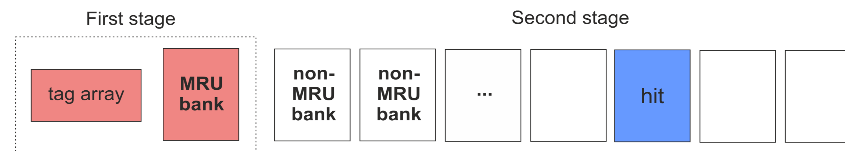
Fig. 3: Diagram of the eDRAM cache access. Pink and blue colors refer to the accessed parts in the first and the second stages (if any), respectively
